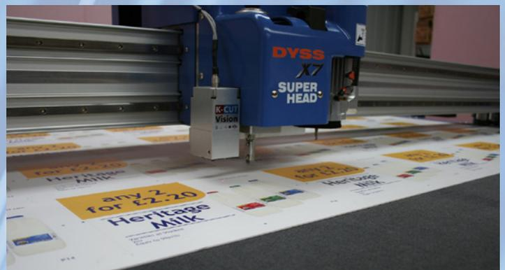
Whilst many of the company's large print runs are cut on a Heidelberg Cylinder, the DYSS has created remarkable efficiencies on its smaller print runs, especially complex boxes and shapes. Recently the company produced 50 presentation folders and 100 bespoke cubes that were printed on the OCE and transferred straight to the DYSS. The boxboard cubes were creased and cut
